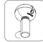
3. Turn the diffuser upside down and insert a 5 mL or 15 mL essential oil bottle into the Bottle Screw-thread. Turn clockwise to tighten. Note: Do not remove the orifice reducer prior to inserting bottle.
